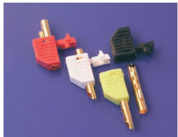
Our **banana plugs** are manufactured using a special beryllium copper sheet and subsequently gold plated. The beryllium gives the copper the necessary spring tension that is needed in order to ensure a high contact pressure when in contact with a socket and therefore guaranteeing security. The acoustic advantages of copper remain largely unaffected.
